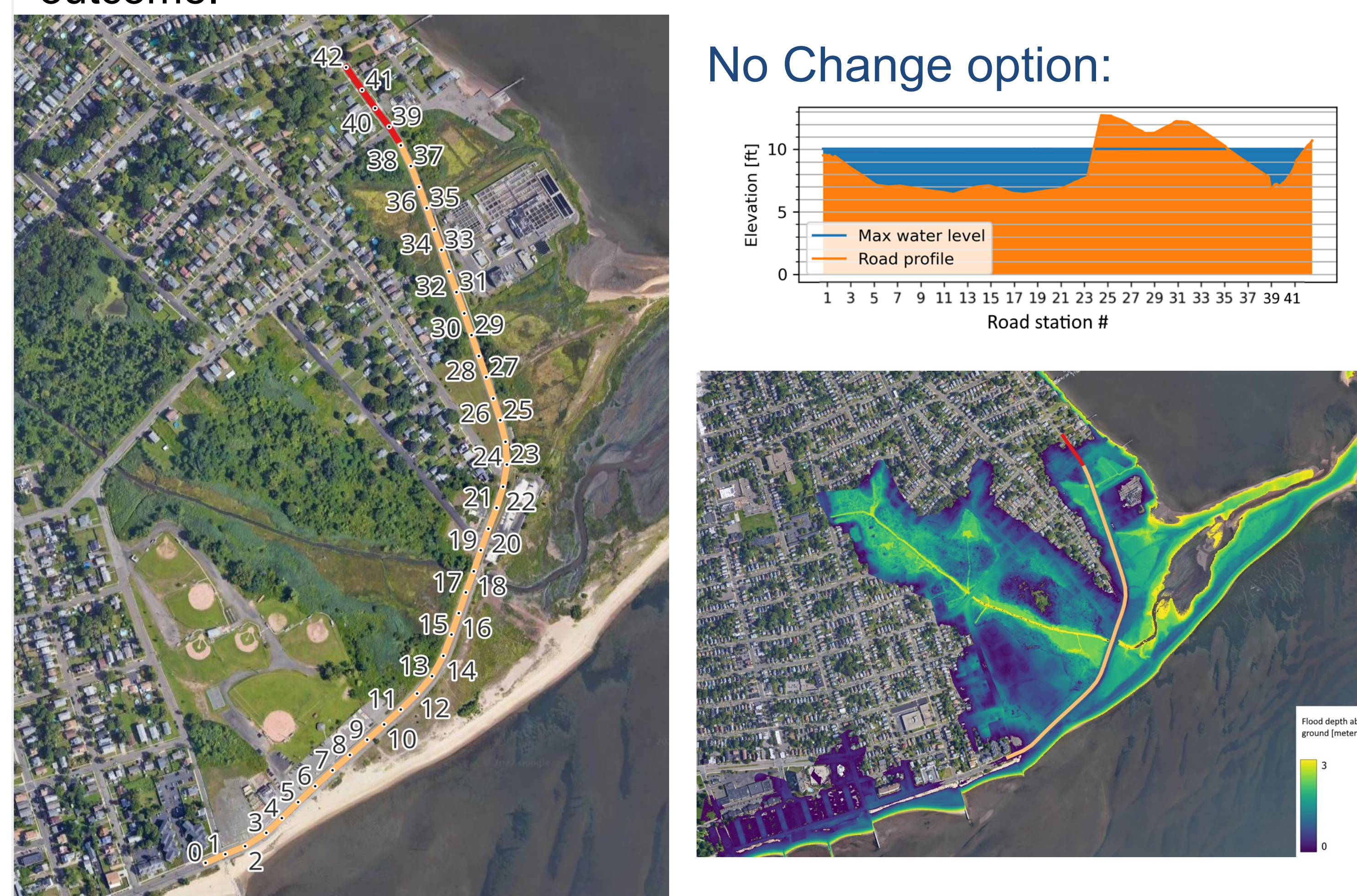
Fig. 2 Left: The portion of 1st Avenue and Beach Street in consideration for raising. Right: Profile of Beach Street and 1st Avenue used in modeling the Current Scenario (upper), and the resulting map of flood depth and extent (lower).
